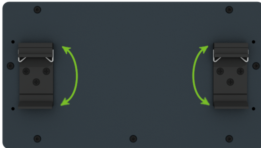
Figure 8: Default Position of the DIN Rail Clips
