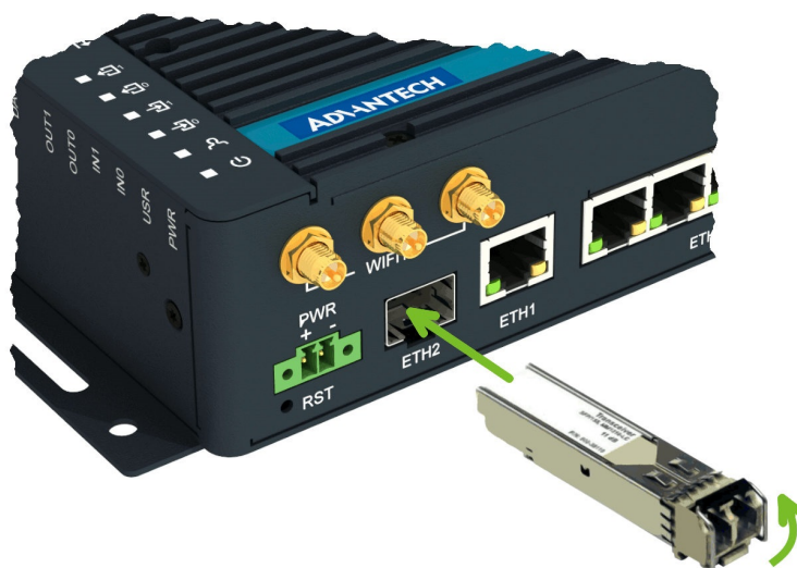
Figure 7: SFP Module Installation
