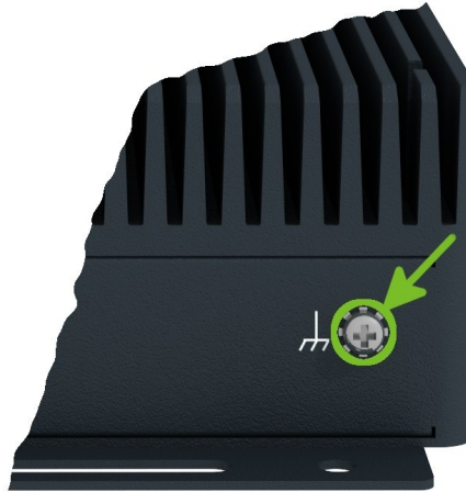
Figure 9: Position of the Grounding Screw
