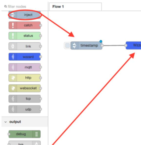
Edit the "inject" node: select JSON as the payload type and enter the string { "pi":30 } to configure a 30 second Publish Interval.
